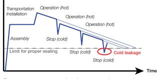
Temperature, pressure and environment are important factors affecting gasket wear and tear. Schedule maintenance at a convenient time before reaching the proper sealing limit.
