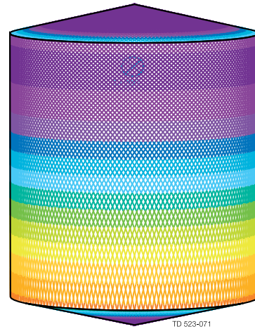
D15 ft H18 ft, Toftejorg TJ 20G, 4 x Ø0.22 inch, Time = 8.3 min, Water consumption = 428 gallon
