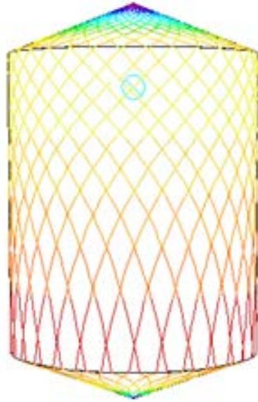
D4.8 m (190"), H7.6 m (300"), 2xØ4.76 mm (2xØ3/16") Time = 2.75 min
