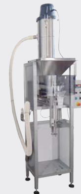
DOSING MACHINE LOAD
